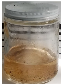
Figure 1- Pictures of Aviation fuel contaminated with dissolved water, dispersed and free water
