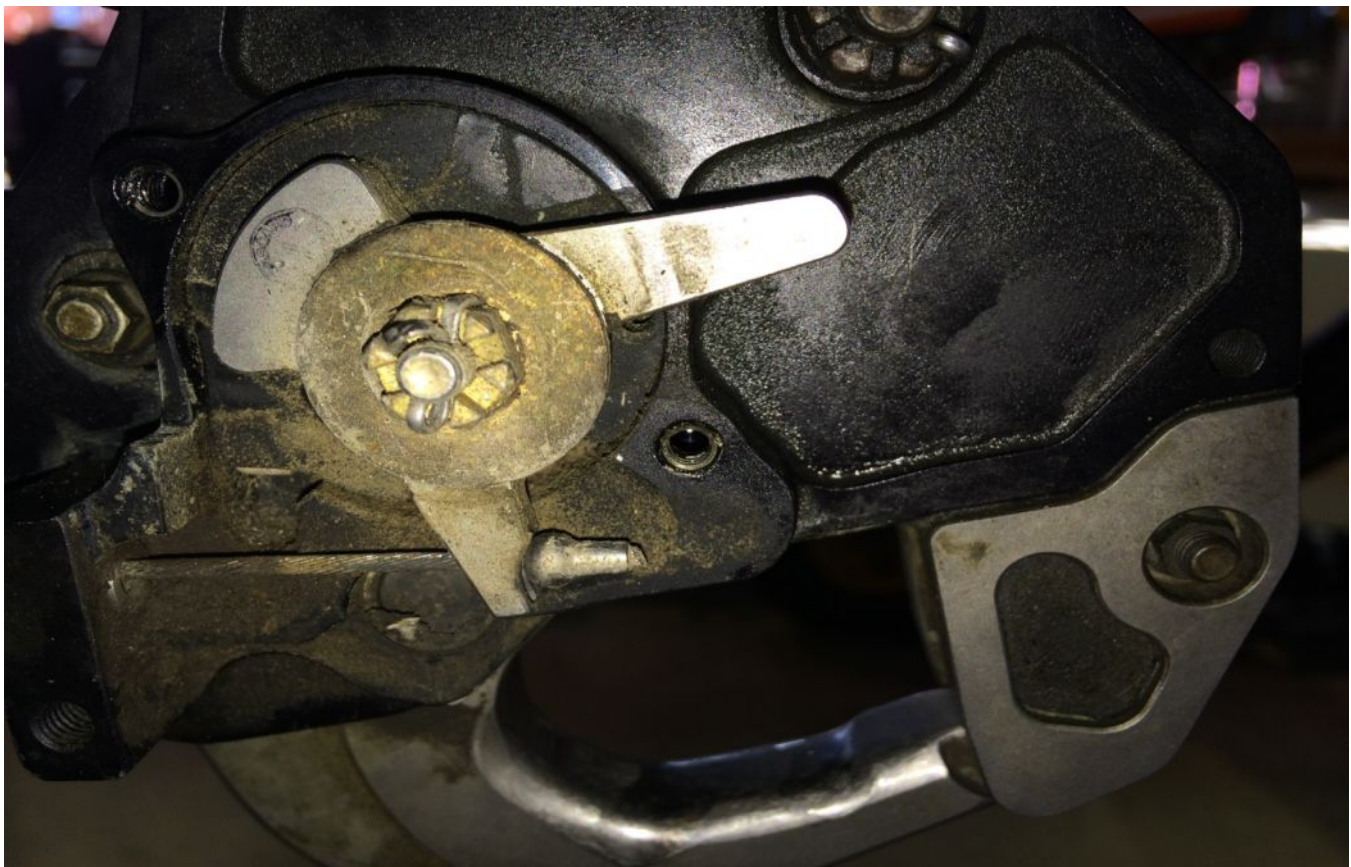
Due to fractured cable conduit, no cable free-play present.
